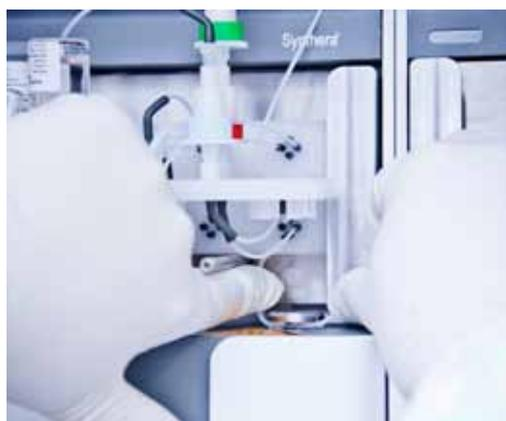
*Synthera® is a multi-purpose automated synthesizer for the production of PET molecules.*
